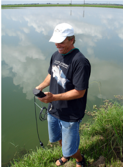
Quick, easy testing with the YSI Pro Plus handheld instrument helps David Maus and his team at Silver Streak Bass Co. stay ahead of ammonium and pH concerns.
