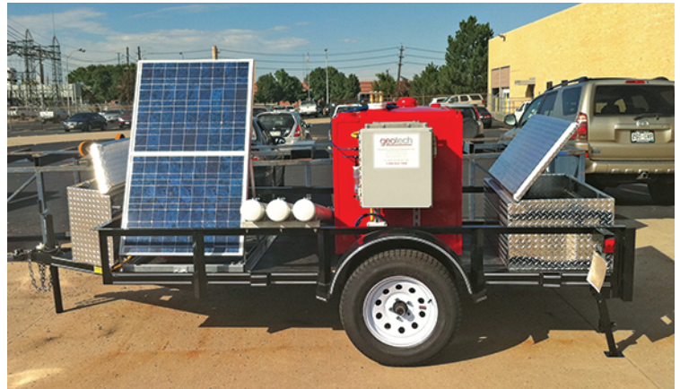
3-Well Solar Sipper on trailer with dual containment tank
