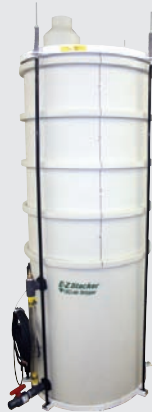
E-Z Stacker® air stripper (U.S. Patent Number 5,518,668)
