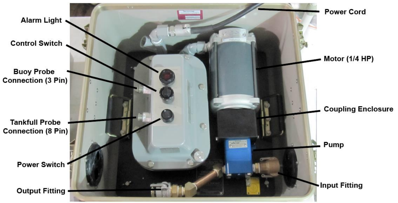
Figure 1-4: New LDFS Pump Control Module Assembly
