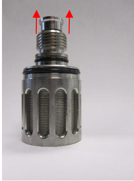
Figure 4-7b: Removing Check Ball Retainer
