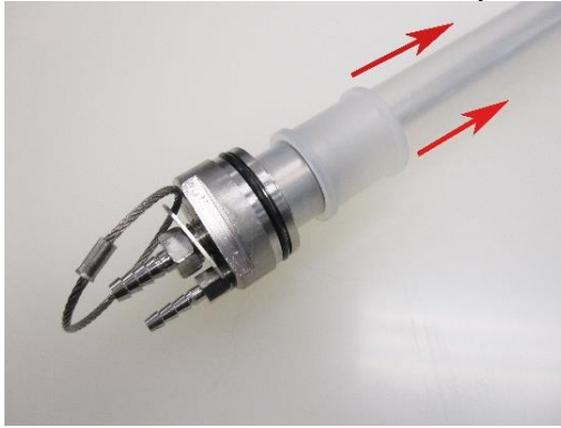
Figure 4-3: Removal of upper Compression Ring
