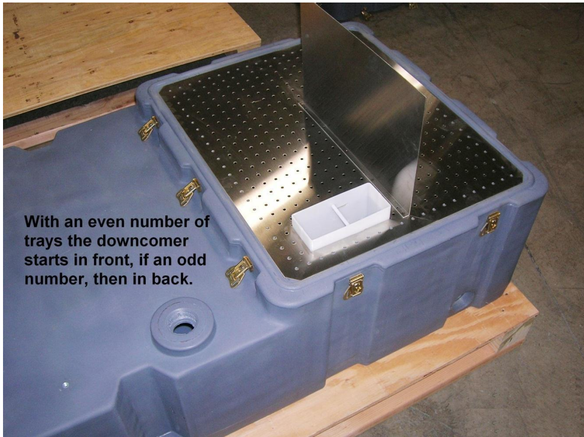
Figure 4-3: First Bubble Plate on Sump
