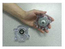
2. Place the tubing around the rollers.
