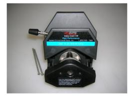
3. Set the lever to the right to close the pump housing onto the tubing.
