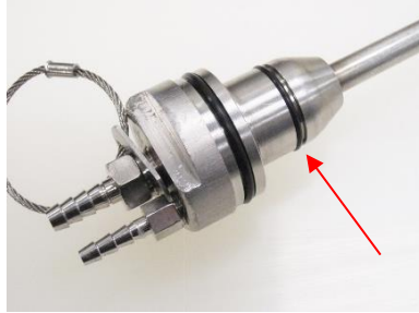
Figure 4-11: Upper end O-ring
