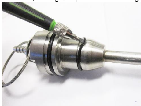
Figure 4-5: Removal of O-rings
