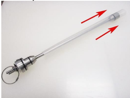
Figure 4-4: Removal of Bladder
