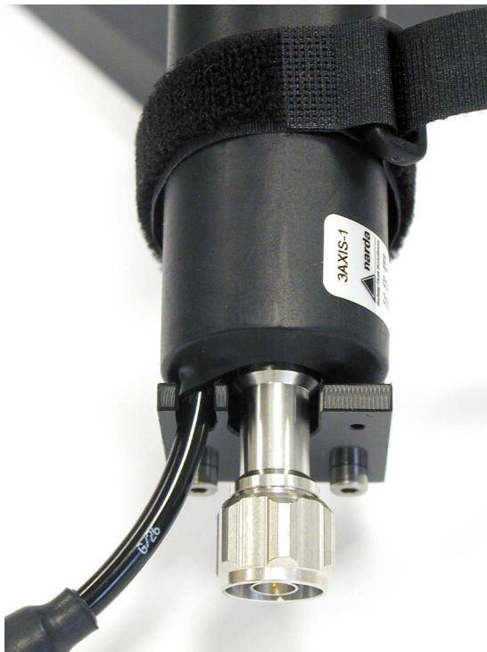
Figure 6: Cable and N connector in guideway
