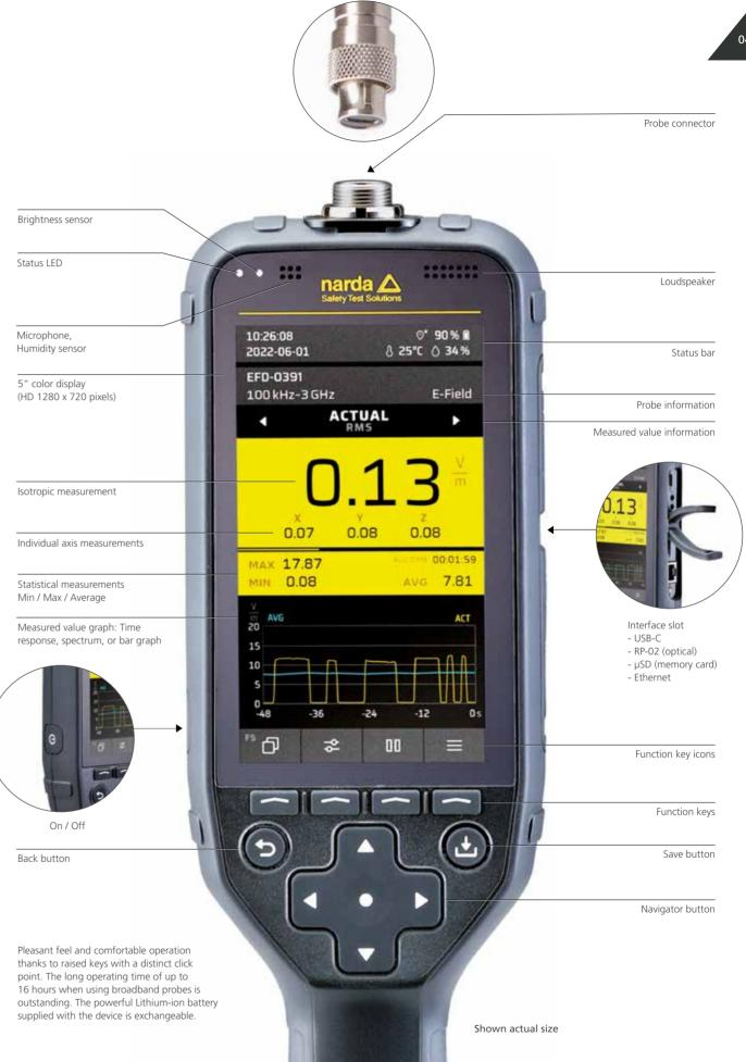
Its compact, handy design and simple operation make the FieldMan the ideal instrument for on-site applications. The sturdy casing and rugged probes ensure reliable results even under adverse weather conditions thanks to IP 54 class protection.
