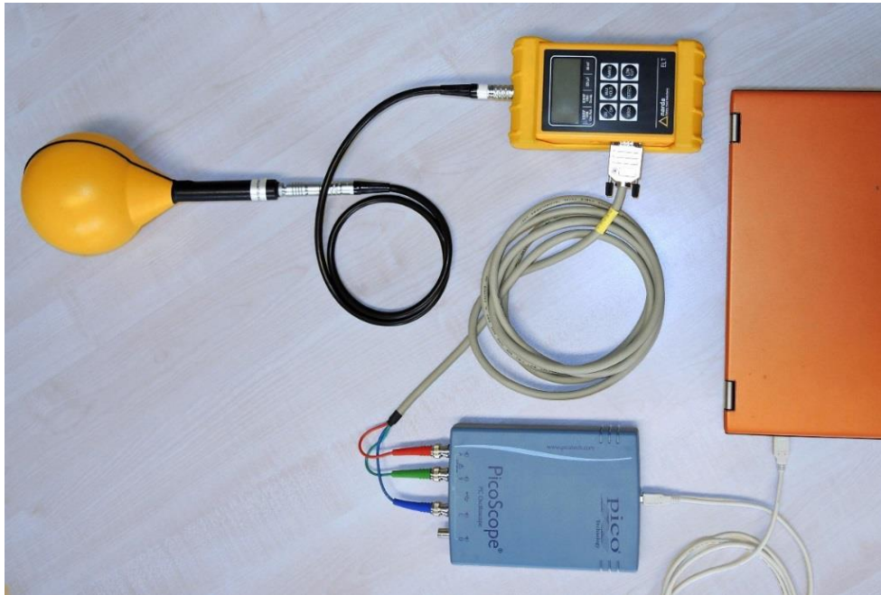
Figure 2: The ELT-400 measuring device with PicoScope 4424 USB data logger and laptop connected
