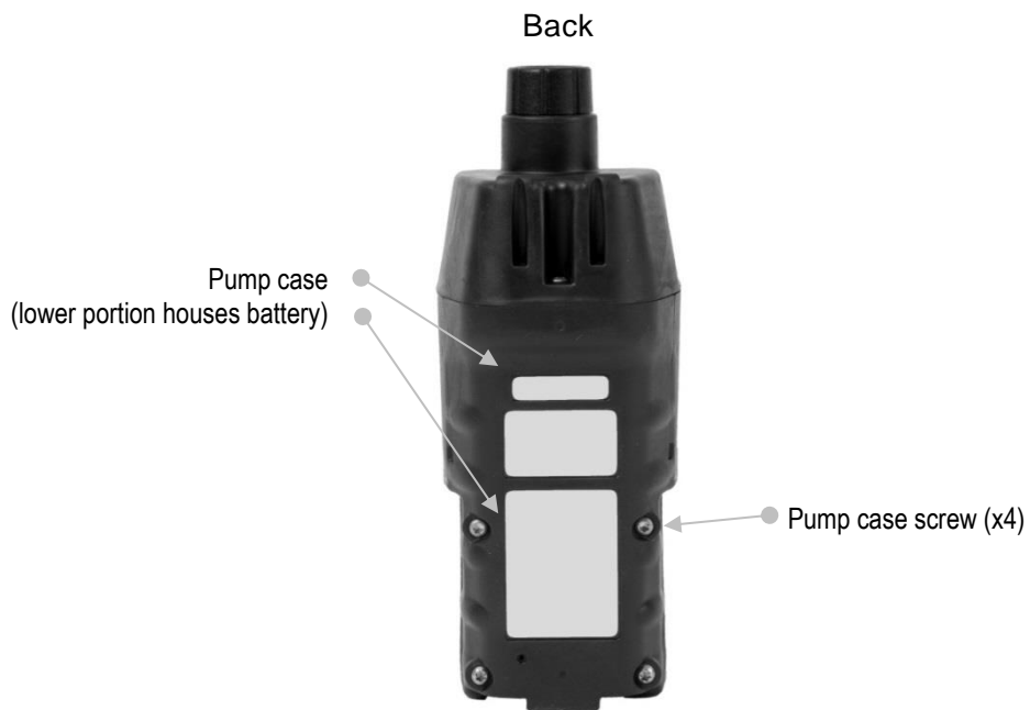
Figure 3.1.B Hardware overview aspirated instrument
