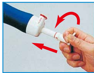
● For more than 200mL sampling, return the handle and repeat procedure ③ and ④.
