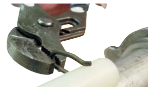
Removing the spring clip allows for easy disassembly of the float.
