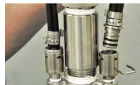
Once the clips are removed, simply pull the connections apart.
