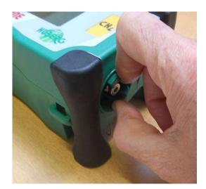
Unlock the filter by turning it counterclockwise and remove it.
