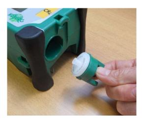
Change the filter and reassemble by turning it clockwise.
