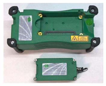
The picture shows the battery pack outside from its compartment.
