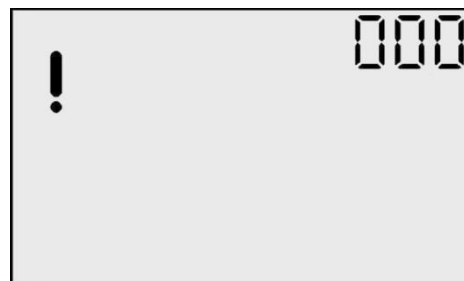
Sensor Missing Error Screen
