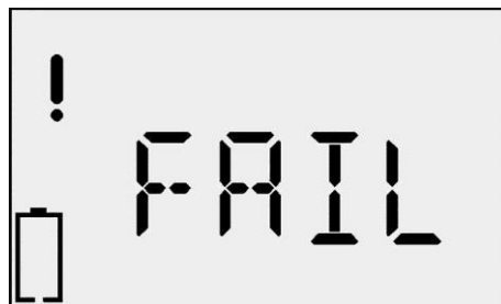
Battery Failure Screen
