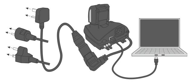
The Cub Doc must be powered on (the Charge LED should be green) for a USB connection to be made.
