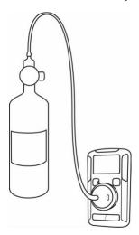
To conduct a bump test, press the button once and wait until the screen displays 985 .
