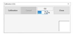
NOTE: Ensure that the Span value is the same as the calibration gas concentration. If not use the Up/Down arrows to adjust (refer to the label on calibration gas cylinder)
