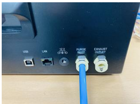
Purge Inlet - 1/8" Tube connect to Clean Air
