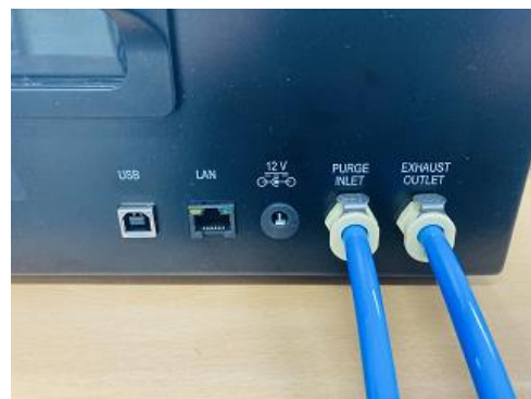
Exhaust Outlet - 1/8" Tube connect to ventilation
