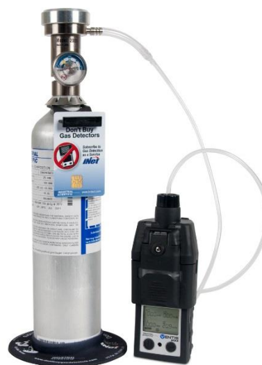
Aspirated monitor with demand flow regulator.
