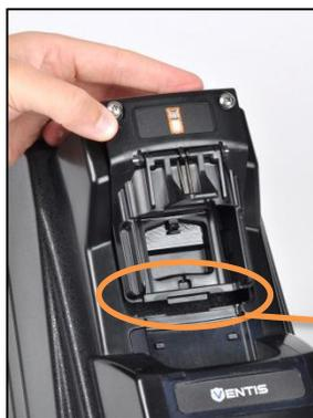
Position the replacement insert's bottom tab into the cutout of the opening; seat into place.
