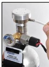
12. Attach the open end of the assembly's tubing to the regulator nipple.
