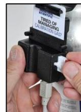
13. If the regulator is equipped with a pressure switch (recommended for DSXi units and required for iNet Accounts), plug its tab into the slot on the side of the card-reader.
