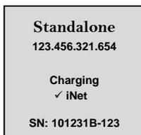
19.1 Find the unit's IP address displayed on the "ready" screen (123.456.321.654 shown here). Open a web browser and enter https:// followed by the unit's IP address and press enter.
