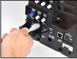
14. Plug the cable connector (arrow faces up) into the iGAS 2 cable port.
