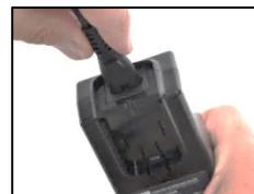
6. In the manner the cover was removed, replace it with the adapter that is suitable for your outlet (above left). If a dedicated power cord was ordered, use it in place of the adapter (above right).
