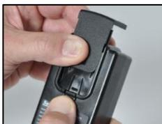
5. From the other end of the power supply, remove its cover: press the release tab and slide the cover in the direction indicated. Store the cover for possible future use.
