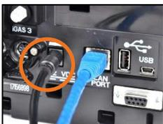
4. Connect the power supply to the docking station's 12 VDC port.
