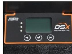
To perform an on-demand, one-button bump test, press the left arrow button (◀). To perform an on-demand, one-button calibration, press the right arrow button (▶). The docking station will ask you to confirm the event and will initiate the respective gas operation after confirmation.
