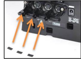
Install the adhesive-backed rubber pads into the recessed areas of the cable retainer.
