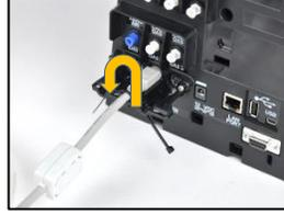
15. From underneath the retaining bracket, insert the narrow tip of the cable tie through the hole to the right of the cable being secured. Feed the cable tie over the cable, then down through the hole on the left side of the cable. Guide the tip through the fastener head.
