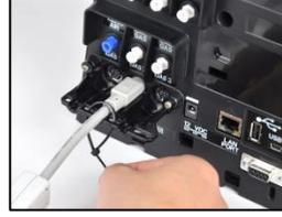
16. Pull the cable tie to tighten the cable securely into position.
