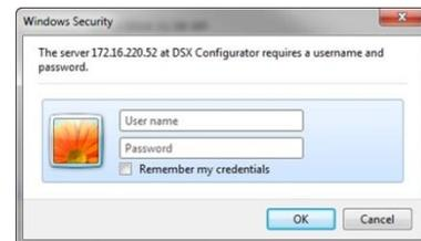
19.3 In the security dialog box, for user name enter DSX, for password enter the unit's serial number (e.g. 101231B-123, case sensitive). Click on OK. You will be prompted to change the password before continuing.
