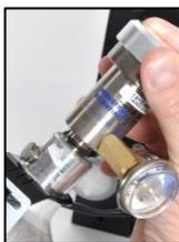
10. Attach the appropriate demand-flow regulator to the cylinder. Turn the cylinder clockwise to tighten.
