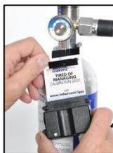
11. Slide the iGas card, which is attached to the cylinder, into the assembly's card reader.
