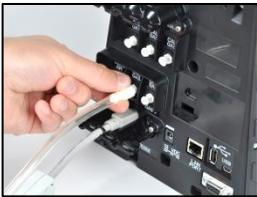
18. Attach the tubing's white swivel connector to the CAL GAS port located directly above the iGAS 2 cable port. Turn clockwise to tighten.
