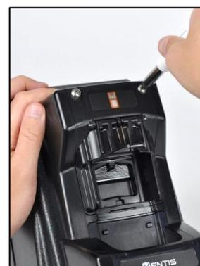
Tighten the top captive screws\* by pushing down to compress the spring, while turning clockwise.
