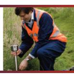
GasClam can be used below ground for up to three months to measure a variety of gases, with temperature, barometric and borehole pressure giving a true long term profile for the first time! It's truly the definitive method of measurement for most below ground applications.
