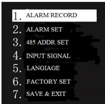
Press the “MENU” button on the normal concentration display interface of the controller to enter the menu. There will be 7 first-level menus: “ALARM RECORD”, “ALARM SET”, “485 ADDR SET”, “INPUT SIGNAL”, “LANGUAGE”, “FACTORY SET”, “SAVE &EXIT”. Press the “UP” or “DOWN” button to select different menu items and press the “MENU” button to enter.
