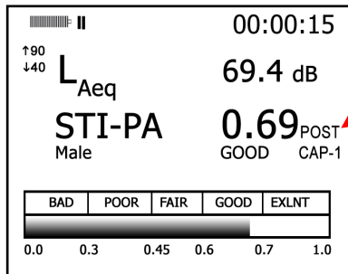
Figure 6-27: Post CAP-1 applied during STI-PA test
