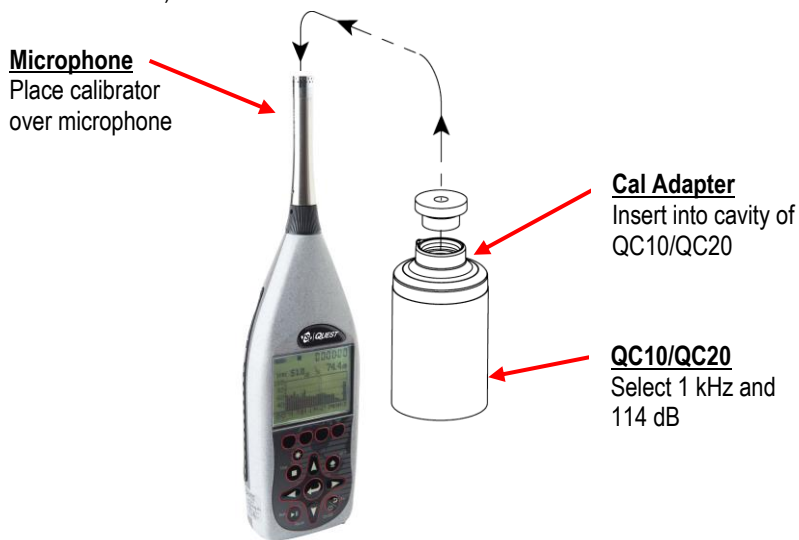
Figure 5-2: Attaching calibrator to SoundPro
