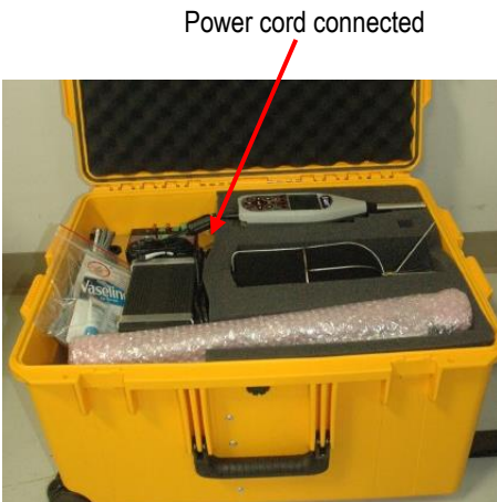
Figure 2: Connecting the battery power
