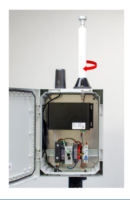
4. Install the TSP head onto the top of the inlet, ensure the inlet's grub screw is loose, and carefully push the TSP head towards the instrument whilst holding the tube adapter still to secure the heated inlet shaft to the tube adapter. Take care not to bend the tubing already secured to the tube adapter.
