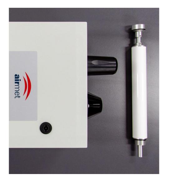
2. Push the inlet into the inlet adapter.
