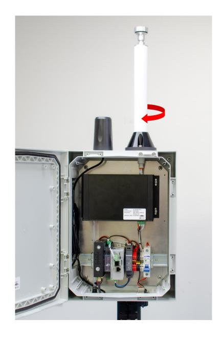
4. Install the TSP head onto the top of the inlet, ensuring that the inlet's grub screw is loose, and carefully push the TSP head towards the instrument whilst holding the tube adapter still to secure the heated inlet shaft to the tube adapter. Take care not to bend the tubing already secured to the tube adapter.
