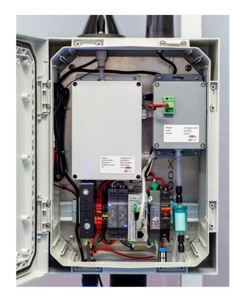
1. Remove the outlet tubing from the particulate sensor module by twisting the luer fitting anticlockwise.
