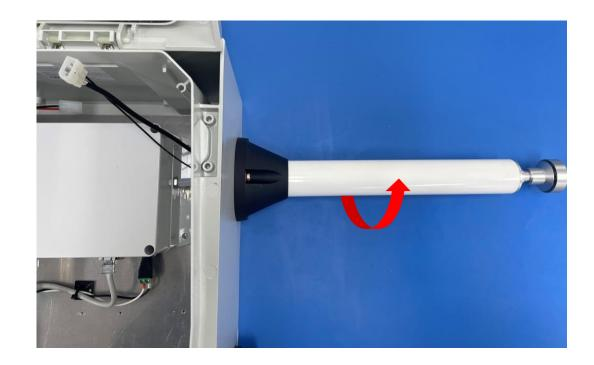
5. Install the TSP head onto the top of the heated inlet, ensure the heated inlet's grub screw is loose, and carefully push the TSP head towards the instrument whilst holding the tube adapter still to secure the heated inlet shaft to the tube adapter. Take care not to bend the tubing already secured to the tube adapter.
