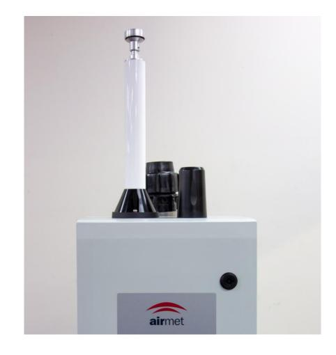
Ensure the O-ring is installed on the heated inlet.
