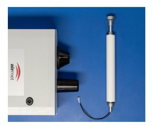
3. Push the heated inlet into the heated inlet adapter and pull the heated inlet cable all the way through the adapter to prevent it getting caught.
