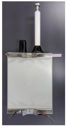
3. Hold the instrument with the mounting rails against the mounting pole of the tripod.
