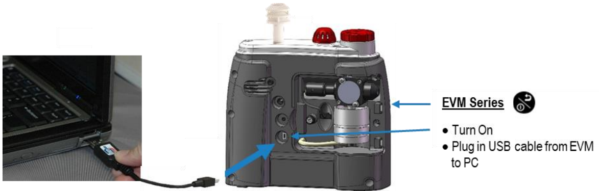
Figure 1-132: Communicating with the EVM and DMS
