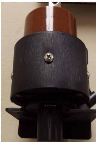
Figure 5-1. CS-7204 being inserted into HD-7204 sensor
