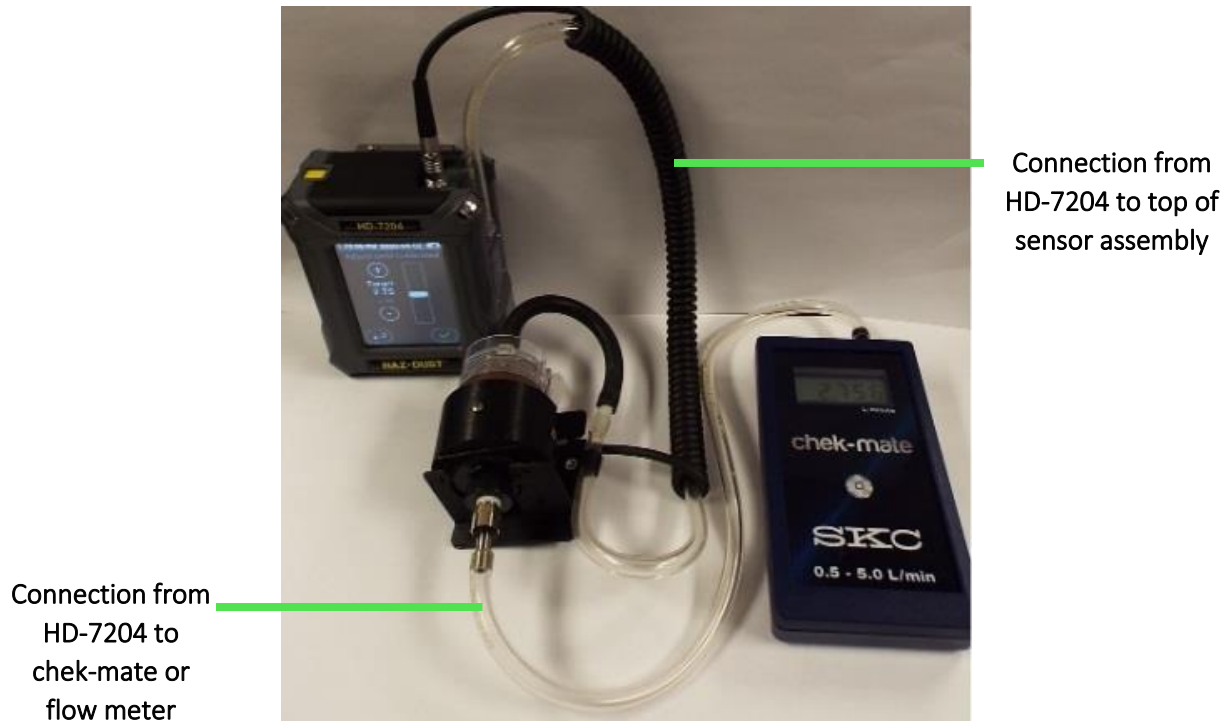
Figure 3-12. Connecting HD-7204 to SKC chek-mate
