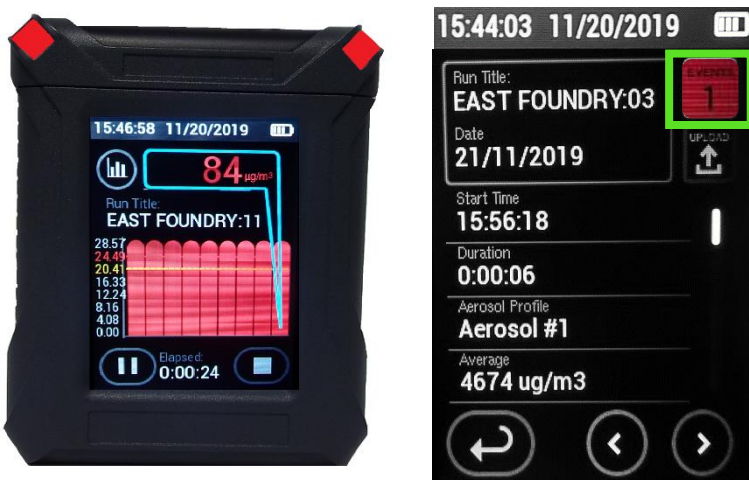
Figure 3-17. Battery Faults cause red lights to flash
