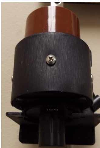
Figure 3-15. CS-7204 being inserted into HD-7204 sensor
