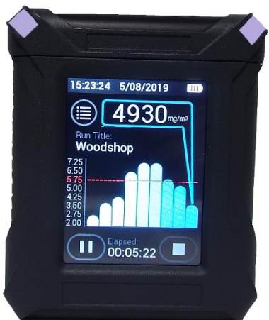
Figure 3-16. Flow Faults cause purple lights to flash
