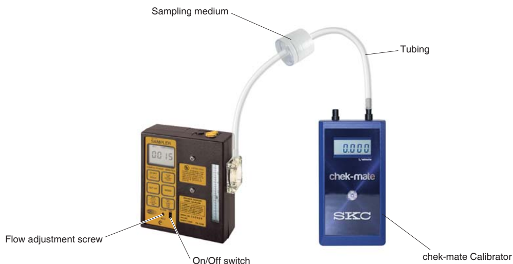
Figure 2. Calibration Train with Filter Cassette
