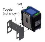
2. Rotate the holder 90 degrees so that the toggle catches securely inside either side of the slot and the bottom plate of the holder is parallel with the bottom of the pump.
