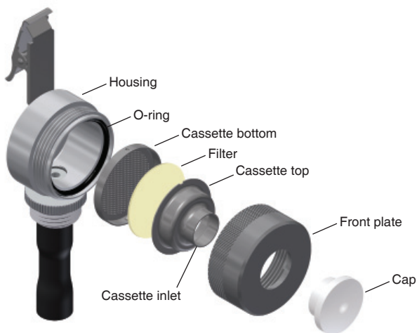
Figure 2. Configuration of Sampling Head and Filter Cassette
