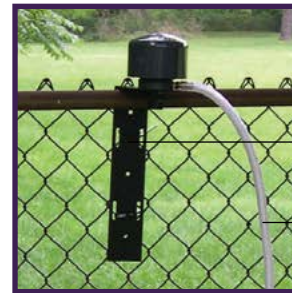
Rain cover protects sampling head
