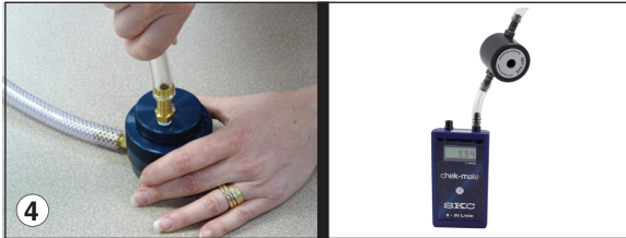
Use a short length of calibration tubing to connect inlet of calibration adapter to outlet of a calibrator to form a calibration train. Note: SKC High Flow chek-mate Calibrator requires Pulsation Dampener Cat. No. 375-150 in line as shown at above right and in Step 5 photo (see Accessories).
