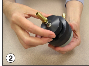
Screw the calibration adapter onto the impactor inlet.
