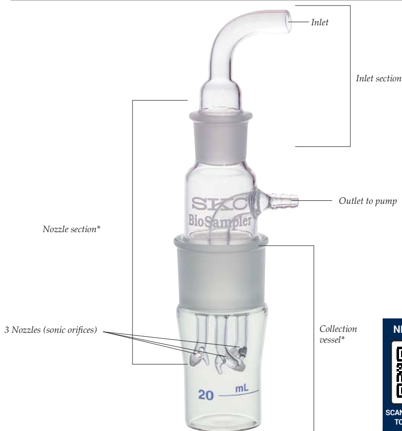
Figure 1. SKC BioSampler Components BioSampler shown with 20-ml vessel (5-ml vessel available)
