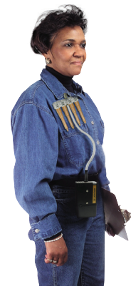
Clip tube holder to worker and pump to belt.
