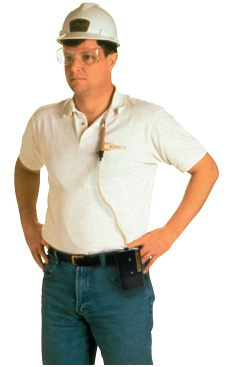
Clip tube holder to worker and pump to belt.
