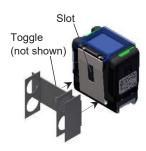
2. Rotate the holder 90 degrees so that the toggle catches securely inside either side of the slot and the bottom plate of the holder is parallel with the bottom of the pump.
