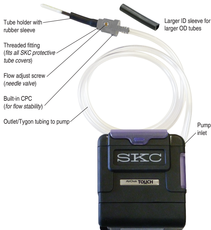
All-in-One Low Flow Adapter/Single Tube Holder with built-in CPC connected to AirChek TOUCH sample pump
