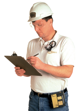
Clip sampling medium to worker and pump to belt.
