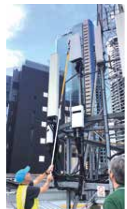
The RF Detection Mode (RadMan 2XT) can be used to quickly and simply check that an antenna has been switched off
