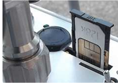
Fig. 4-10 SIM card installation
