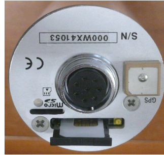
Fig. 4-13 SIM card installation
