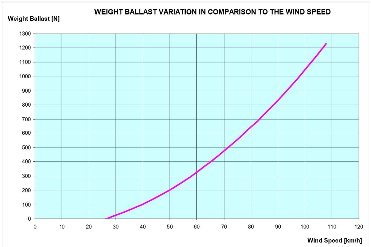
Fig. 7-4 Weight Ballast variations in comparison to the wind speed for AMB-8059/01 and AMB-8059/03 with joint
