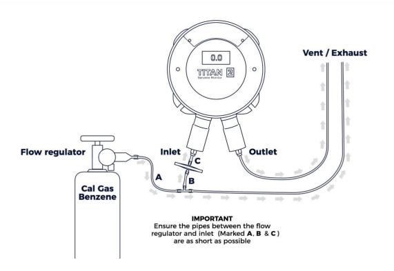
If the Titan 2 does not display the gas concentration given by the bottle, calibrate the Titan 2 to give the correct readings. Refer to:
