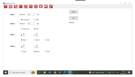
You can set each alarm to operate when the STEL or Current level of Benzene reaches a set value in ppm.
