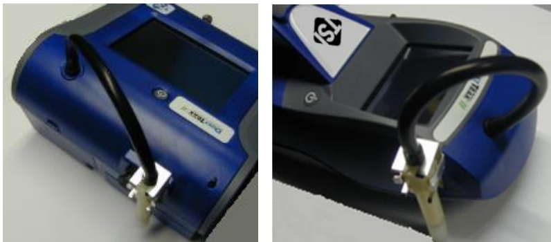
Figure 2-8: Installing Door-Oliver Cyclone
