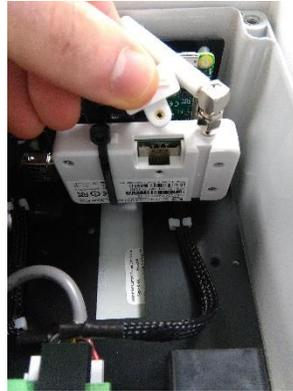
**2** Rotate modem aerial up to access the SIM card cover (the retaining screw is removed in the factory). Slide the cover up to remove it.
