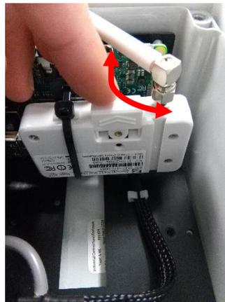
**4** Rotate the aerial back to the horizontal. When replacing the front cover ensure the vent is at the top with the opening facing down.
