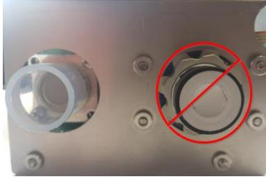
4 Never directly touch the exposed NO<sub>2</sub> sensor at the bottom. If for any reason the sensor becomes disconnected from your replacement sensor assembly only grip the sides of the sensor when reconnecting.
