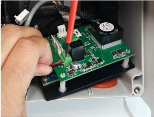
5 Connect the positive and negative power supply cables to the replacement O<sub>3</sub>/NO<sub>2</sub> sensor module. Ensure you double check the polarity
