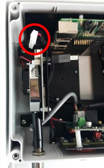
❸ Disconnect white connector at the top of the PM sensor.
