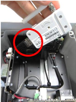
3 Connect the modem to the AQY 1 using the USB connection as shown above. Position the modem against the vertical upright with the pointed end of the cable tie extending out on the top side.
