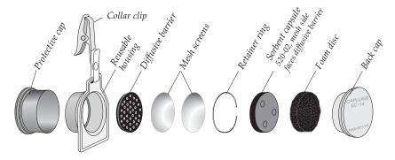
Figure 1. Complete Assembly of Passive Sampler for Elemental Mercury
