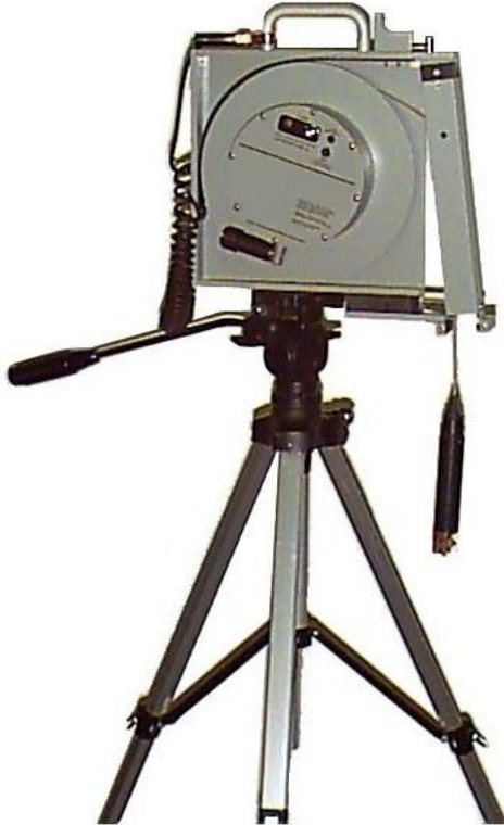
Figure A-1: Example of Interface Probe Assembly mounted to tripod
