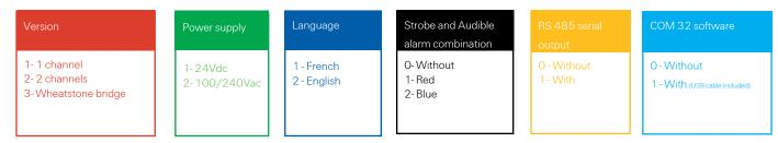
f.i: MX32-1-2-2-1-1 for MX32 1 channel, 100/240Vac, English, Blue strobe & horn, RS485 output et COM 32 software
