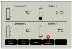
1Up to eight detectors displayed simultaneously
