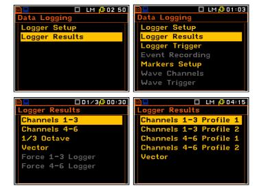
In **Advanced Mode** it is possible to define logger results for each channel and profile individually.
