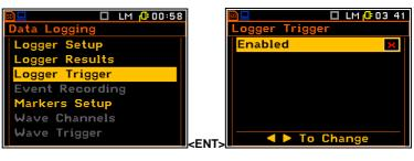
The logger triggering of the measurements (**Enabled**) can be switched on by means of the < > > push-button.
