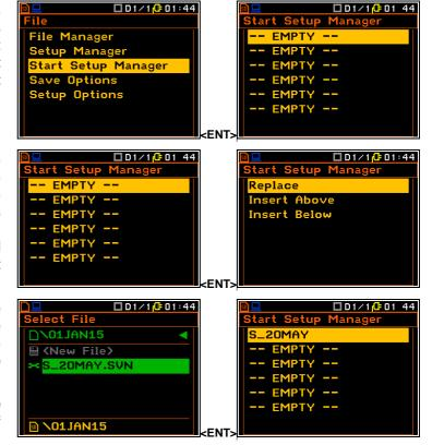
In case of pressing the **<ENTER>** pushbutton on an existing assignment, the **Remove** option will also be available. Please use it to remove the assignment. The setup file itself will not be removed.
