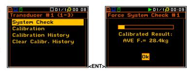
After entering the **Calibration** option, user will be asked to press SV 105AF sensor with hand straps against a scale so that this scale indicates between 18 and 20 kg.
