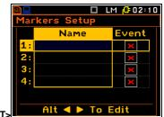
window that is opened by means of the < ◀ >, < ▶ > push-buttons pressed together with <**Shift>** or <**Alt>** while the cursor is on the **Name** position.
