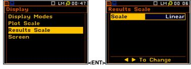
There are two options for the **Scale** parameter: **Linear** and **Logarithm**. In the case of **Linear** all the results are shown in linear units. In case of **Logarithm** the measurement results are expressed in decibels (the results are related to the values set in the **Reference Level** window (path: <Menu> / Auxiliary Setup / Reference Levels).
