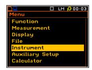
The **Instrument** list content depends on **Instrument Mode** selection from the **Auxiliary Setup** menu: **Simple Mode** or **Advanced Mode**.
