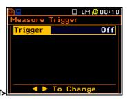
The **Measure Trigger** is a contexts sub-list in which the triggering can be switched off or on (**Trigger**), when on it can be determined the source of the triggering signal (**Source**), the channel of source signal (**Channel**), its level (**Level**) and sometimes also the speed of changes (**Gradient**). If **RTC** is selected as trigger type, start time (**RTC Start**) and repetition of triggering (**Repeat Every**) is defined.
