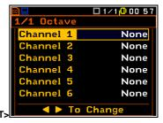
If the **None** value is selected in the **Channel x** position then spectrum data will not be saved in the logger file. If **RMS** value is selected, then RMS spectrum will be saved in the logger file for this channel.
