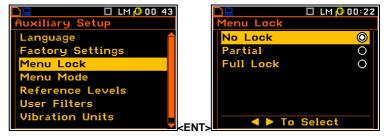
The activation of **Partial** results in locking access to the **Menu** options, which are responsible for measurement parameters. In the case of **Full Lock** no one position from the **Menu** lists is accessible and after attempt of enter **Menu** the **Menu Lock** window appears on the display. The **Menu** is available after unlocking it.
