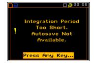
When the **Auto Save** option is active, after starting the measurements by pressing the **<Start/Stop>** push-button the results are saved in the file with the selected name.
