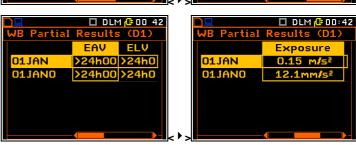
When **Simple Mode** function is selected in the **Instrument Mode** sub-list, then **Vibr. Dose Calculator** list consists of the first three positions only.
