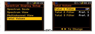
By default **HP** filter is denote for the first Total value. Second and third Totals have same filters as were set up for profiles (**Prof. 1** and **Prof. 2**) in the **Channels** window (*path:* <*Menu>* / *Measurement* / *Channels*).
