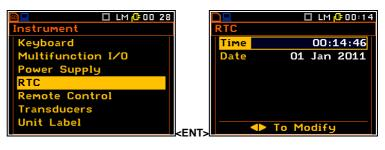
Editing the time is performed in the special window, which is opened after pressing the  $<^{\flat}>$  push-button. The selection of the correct parameter (hour, minute, second, and also day, month and year) is performed using the  $<^{\blacklozenge}>$ ,  $<^{\flat}>$  push-buttons and the change of its value – using the  $<^{\spadesuit}>$ ,  $<^{\blacktriangledown}>$  push-buttons pressed together with <Alt>.
