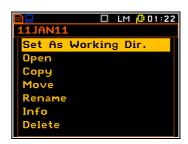
There are two options for storing result data in the internal or external memory. One option is to press **<Save>** push-button immediately after the measurement. Another option is to create **<New File>** in the **File Manager** window.
