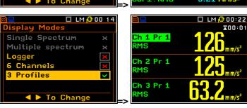
When all display modes in the **Display Modes** list are switched on they all are available and can be selected by means of the Alt> and A>> push-buttons.
