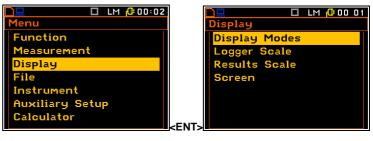
The **Display** list is used for setting the various parameters, which are mainly dedicated for the control of the screen display views. The list consists of:
