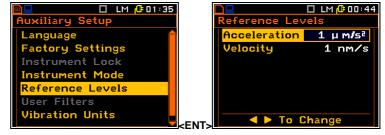
In the **Acceleration** position the user can set the reference level of the acceleration signal from  $1 \mu ms^{-2}$  to  $100 \mu ms^{-2}$ . In the **Velocity** position the user can set the reference level of the velocity signal. It is possible to set this level from  $1 nms^{-1}$  to  $100 nms^{-1}$ .
