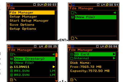
The files are saved in the Memory and in the catalogue which was set up as the working directory. The working Memory type is displayed as the icon in the left position of the icon line.
