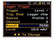
triggering condition. The level of the triggering source can be set in a range from **60 dB** to **200 dB** or from **1.00 mm/s**<sup>2</sup> to **10.0 km/s**<sup>2</sup>, depending on what scale type was selected in the **Scal**e position (*path:* <*Menu> / Display / Results Scale*).
