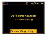
If there are conditions to execute the **Defragmentation** operation the current progress of defragmentation is shown on the display. After successful defragmentation, the special message is displayed and the instrument waits for the reaction of the user. Any push-button should be then pressed except **<Shift>** and **<Alt>**. After pressing a push-button, the instrument returns to the **Defragmentation** sub-list.
