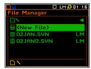
The list of operations on files saved in the **Internal** memory differs from **SD Card** by one position. It is not possible to rename the files saved in the **Internal** memory and thus the **Rename** position in this list is not active.
