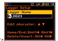
The edited name is accepted and saved after pressing **<ENTER>**. The special warning is displayed in case a file with the edited name already exists in the memory. The instrument waits then for a reaction of the user (any push-button should be pressed except **<Shift>** or **<Alt>**).
