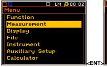
The Measurement list and some of sub list (General Settings and Data Logging) contents depend on Instrument Mode selection from menu Auxiliary Setup: Simple Mode or Advanced Mode. In Advanced Mode some additional functions like triggering, markers, event and wave recording appear.
