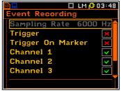
When the **Trigger** position is selected then event recording will start by trigger.
