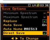
The **Setup Options** sub-list is used for the selection of the options for storing setup files.
