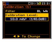
The measurement starts after 5 seconds delay. The calibration measurement time is also predefined to 5 seconds. During the calibration period the **<ESC>** and **<Pause>** push-buttons do not operate but it is possible to stop the measurement using the **<Start/Stop>** push-button. Waiting for the calibration measurement to begin, a **Delay** is counted down. At the end of the measurement, its result is displayed on the display in the bottom line.
