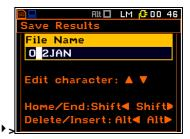
The edited name is accepted and the instrument returns to the **Save Results** window after pressing **<ENTER>**. Pressing the **<ENTER>** push-button again saves the file in the working directory. The special warning is displayed if a file with the same edited name already exists in the memory. The instrument waits then for a reaction from the user (any push-button should be pressed except **<Shift>** or **<Alt>**).
