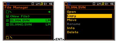
In order to perform this operation select the file/catalogue and press the **<ENTER>** push-button. After opening the list of operations select the **Copy** position and press the **<ENTER>** push-button again. The instrument then will propose to choose the target catalogue for copying. After selection of the target catalogue the user should press the **<ENTER>** push-button. The window with two options will appear: **Copy Here** and **Rename**.
