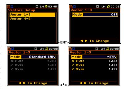
When the user needs to calculate a vector with other than standard coefficients, it is possible to select the coefficient within the values from **0.00** to **2.00**.
