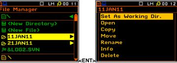
When **SD Card** is selected the first two positions **<New Directory>** and **<New File>** can be used to create new elements. When **Internal** memory is selected only the **<New File>** position is available.
